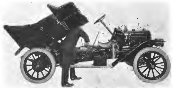
Motor Accessibility on the Two-cylinder Rambler.
